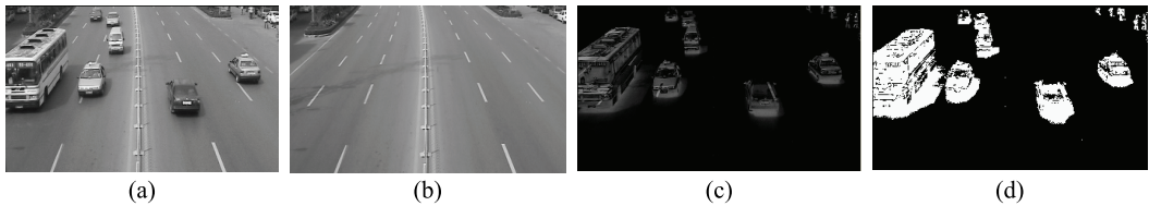
Fig. 7. The process of extracting the moving object area: (a) the current input image, (b) the generated background image, (c) the difference image, and (d) the binary difference image.
