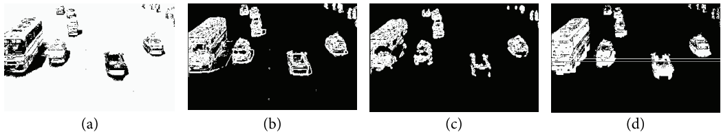
Fig. 8. The processes of elimination of moving cast shadows: (a) the pre-extraction of the cast shadows, (b) the binary edge image, (c) the elimination of the cast shadows edge pixels, and (d) the binary image of object areas.
