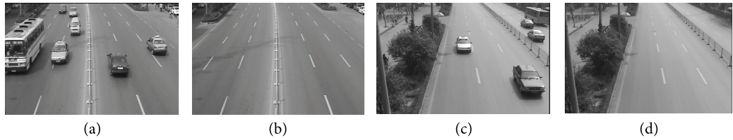
Fig. 5. Background extraction effect for different scenes: (a) foreground of scene 1, (b) background of scene 1, (c) foreground of scene 2, and (d) background of scene 2.
