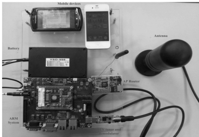
Fig. 7. System testing prototype.
