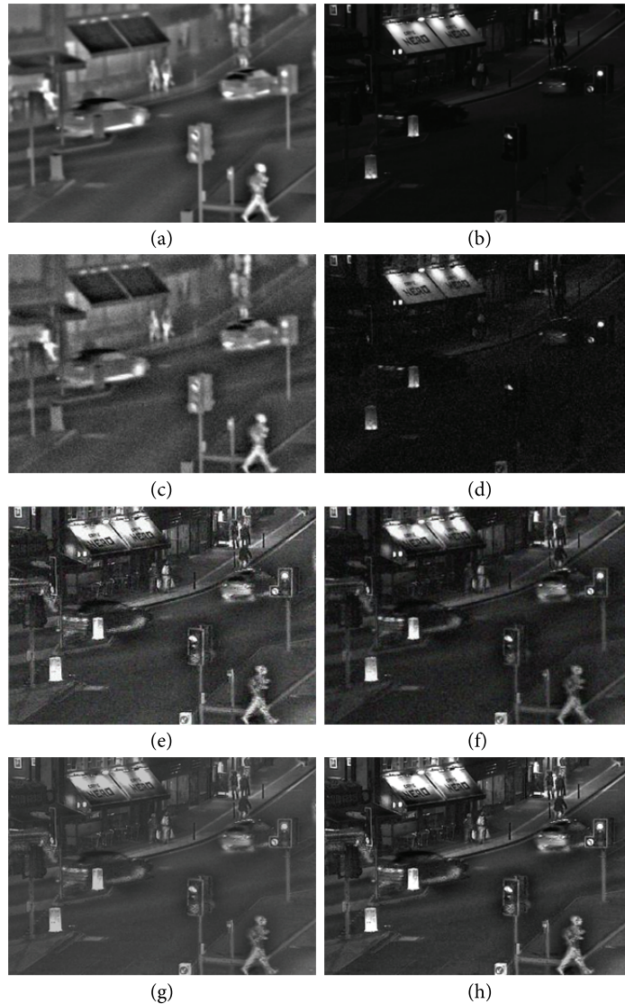
Fig. 7. Comparison of various fusion methods' effect (Bristol Queen's Road image). (a) Infrared image, (b) visible image, (c) adding noise infrared image, (d) adding noise visible image, (e) NSCT method, (f) shearlet method, (g) DBM-DWT method, and (h) proposed method in this paper.
