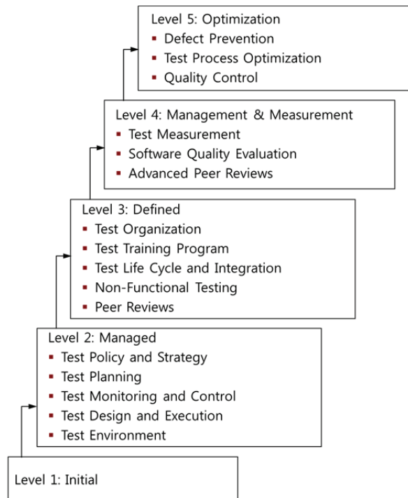
Fig. 1. Test Maturity Model integration (TMMi) model.
