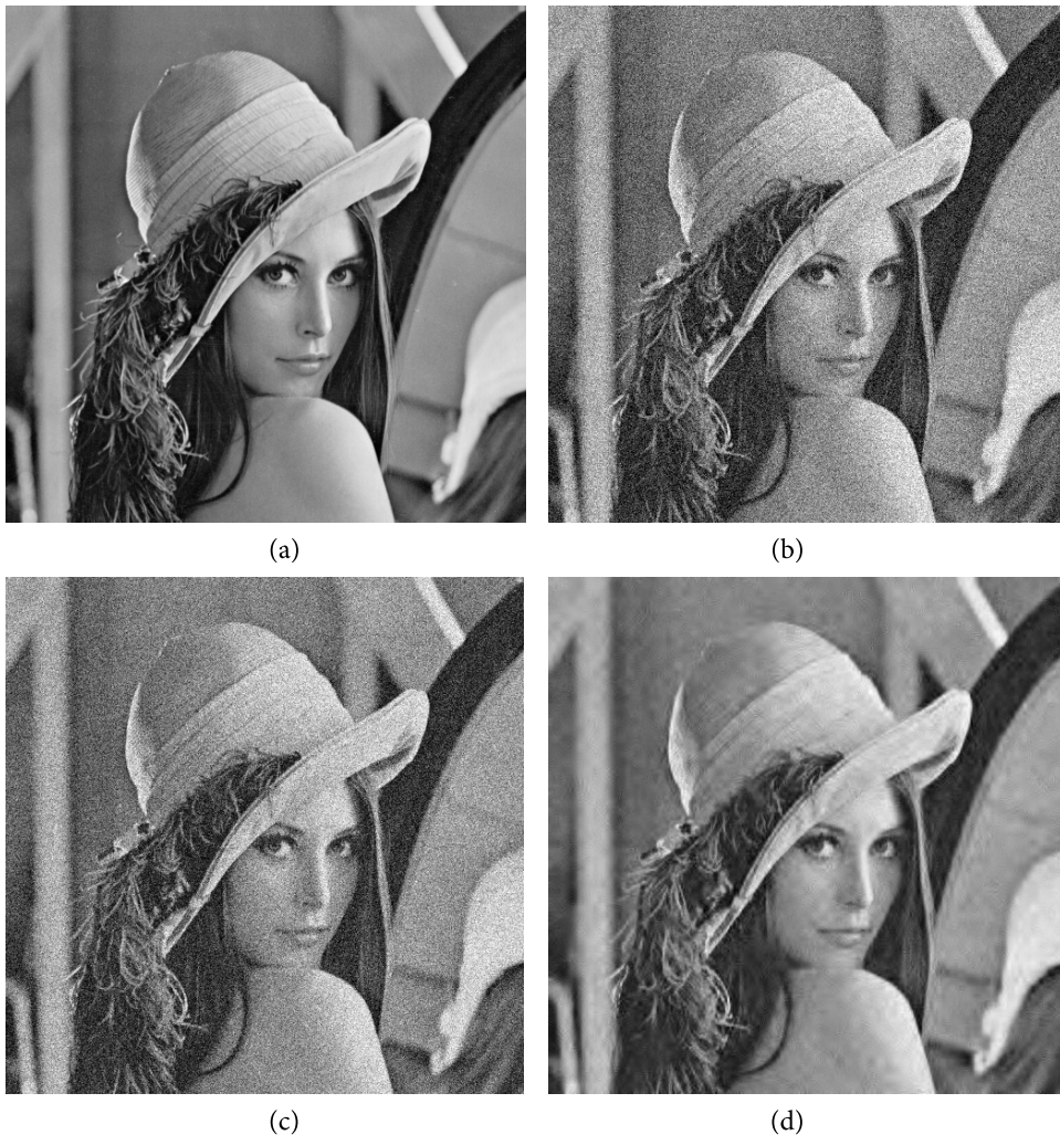
Fig. 2. Effectiveness of denoising the Lena image contaminated with Gaussian noise: (a) original image, (b) noisy image, (c) improved AMF, and (d) GMM algorithm.
