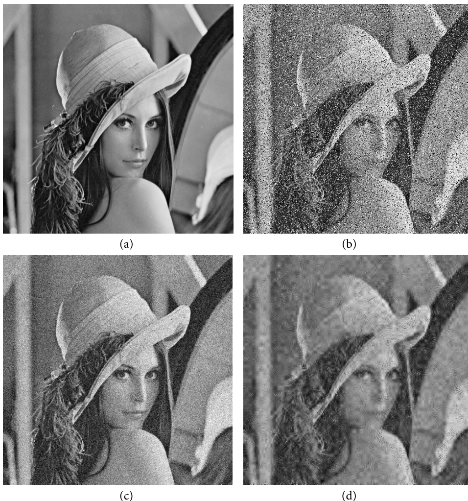
Fig. 3. Effectiveness of denoising the Lena image contaminated with mixed noise: (a) original image, (b) noisy image, (c) improved AMF, and (d) GMM algorithm.
