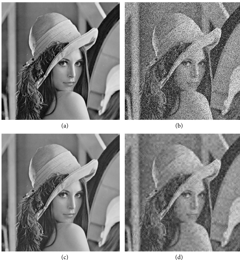
Fig. 1. Effectiveness of denoising the Lena image contaminated with impulse noise: (a) original image, (b) noisy image, (c) improved AMF, and (d) GMM algorithm.
