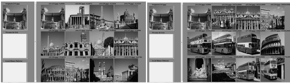
Fig. 10. Results obtained by querying with image #232 (Class: Building). (a) GLIBP (precision=12/12) and (b) LBP (precision=7/12).
