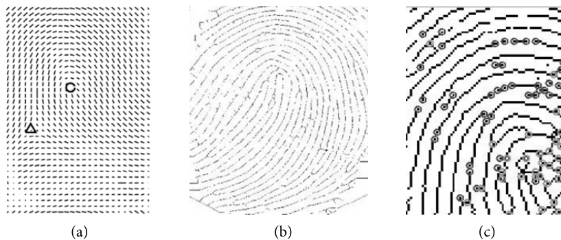
Fig. 3. Fingerprint with directional field, singular points, skeletonization, and minutiae. (a) Directional field and singular point. The core is indicated by the circle and the delta by the triangle. (b) Skeletonization of a segmented fingerprint. (c) Minutiae extracting: end ridge in red and bifurcation in green.
