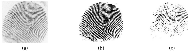
Fig. 4. Segmentation: (a) original fingerprint, (b) fingerprint segmentation with Otsu, and (c) fingerprint segmentation with global thresholding.
