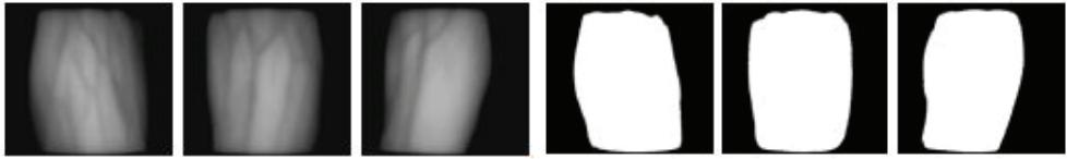
**Fig. 4.** Binarization for hand area extraction.
