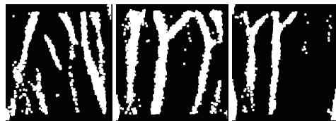
**Fig. 9.** Vein binary image after dilatation window (7×7).
