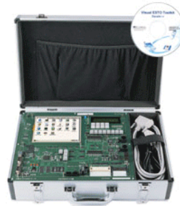
Fig. 9. Embedded board and expansion kit
