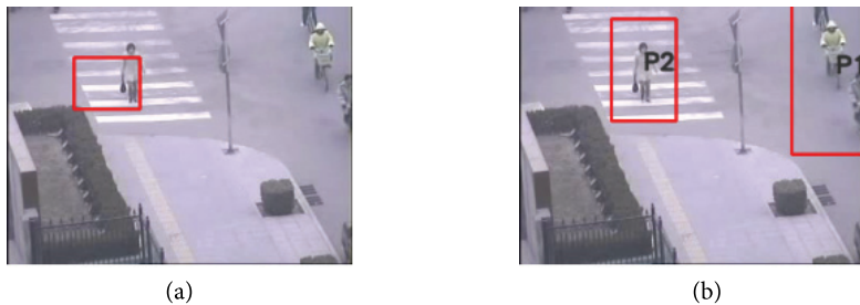
Fig. 13. Correction of tracking error 2: (a) partial-mapping error by SURF tracking and (b) correction by the proposed tracking.
