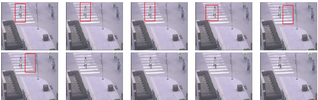
Fig. 17. SURF tracking [8] with an incorrect-mapping error in the top-right to bottom-left direction.
