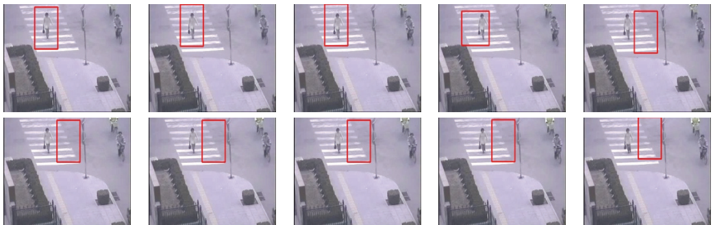
Fig. 20. Meanshift tracking [9] to correct the tracking error in Fig. 17.
