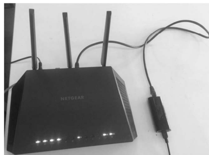
Fig. 5. The applied router and the smart gateway for connecting the air conditioners to the Internet.
