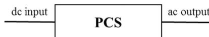
Fig. 3. Inverter mode of the PCS for evaluating the DC to AC power conversion efficiency.
