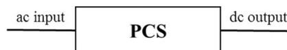
Fig. 4. Converter mode of the PCS for evaluating the AC to DC power conversion efficiency.
