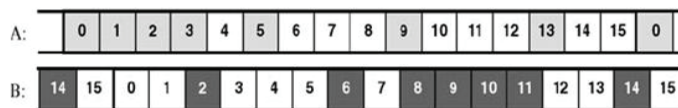
Fig. 2. Sleep/wakeup periods of quorum-based system and nodes overlapping (awake BIs are shown by dark color) [14].
