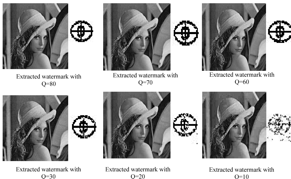
Fig. 12. The extracted watermark from Lena image after different values of quality factor (Q).
