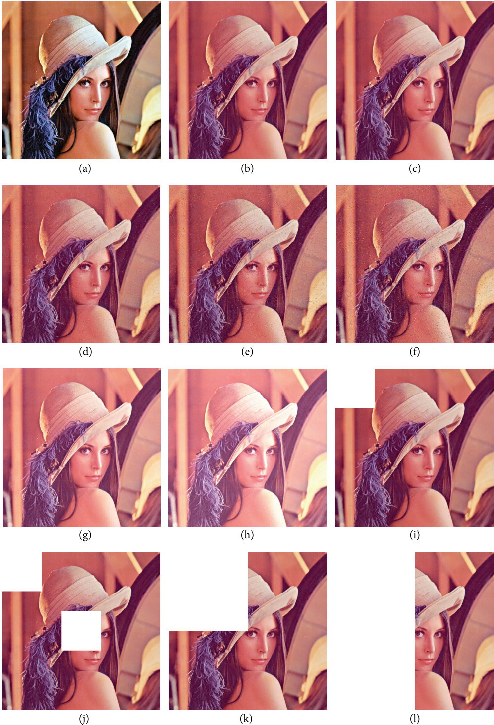
Fig. 7. Watermarked images after adding different kinds of attacks: (a) contrast adjustment (default), (b) JPEG compression (QF=90), (c) JPEG compression (QF=95), (d) salt and pepper noise (0.01), (e) salt and pepper noise (0.02), (f) salt and pepper noise (0.03), (g) Gaussian noise (0.1), (h) Gaussian noise (0.2), (i) cropping (1/16), (j) cropping (1/8), (k) cropping (1/4), and (l) cropping (1/2).
