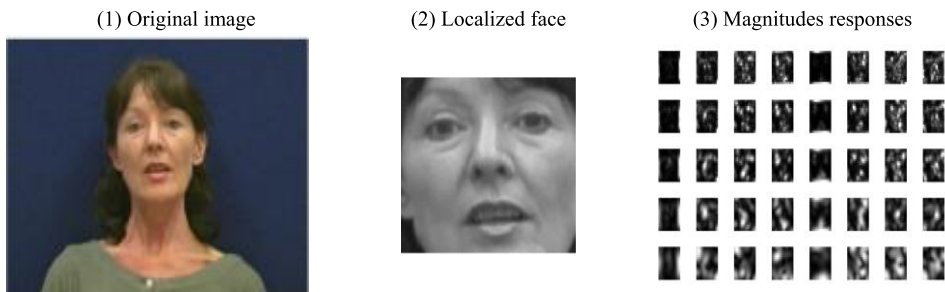
Fig. 2. Magnitude responses of the filtering operation with the Gabor filter bank (no down-sampling) using the 1st subject image in VidTIMIT database.
