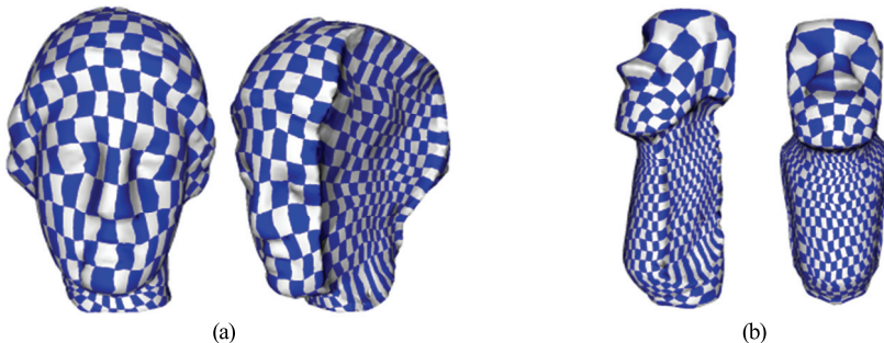
Fig. 4. Cubic volume parameterization results: in (a) and (b), the figures on the left show the boundary condition \partial\phi while those on the right depict the result of cubic volume parameterization \phi by visualizing the part corresponding to \{(s, t, u) \mid 0 \leq t, u \leq 1 \text{ and } 0 \leq s \leq 0.8\}
