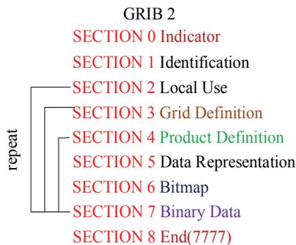
**Fig. 2.** GRIB2 encoding format.
