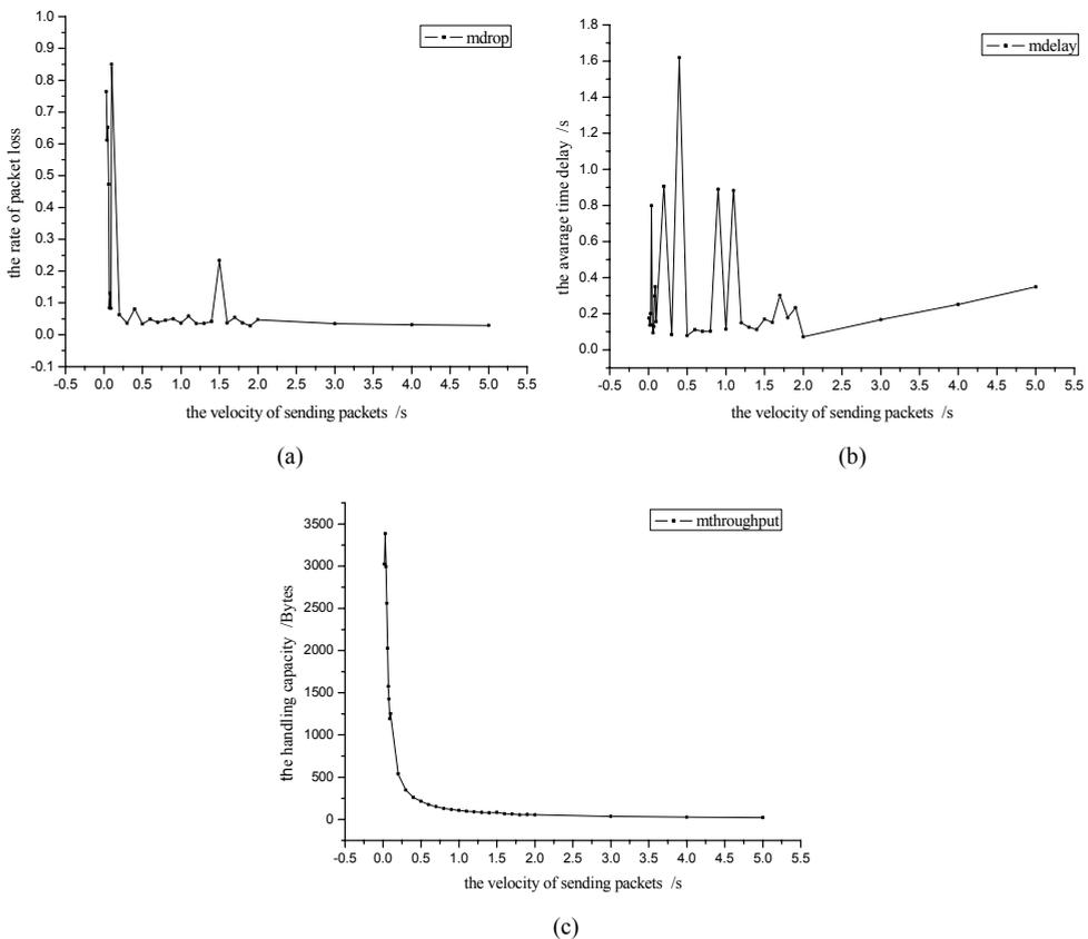
Fig. 6. Performance graphs of the multi-hop communication
