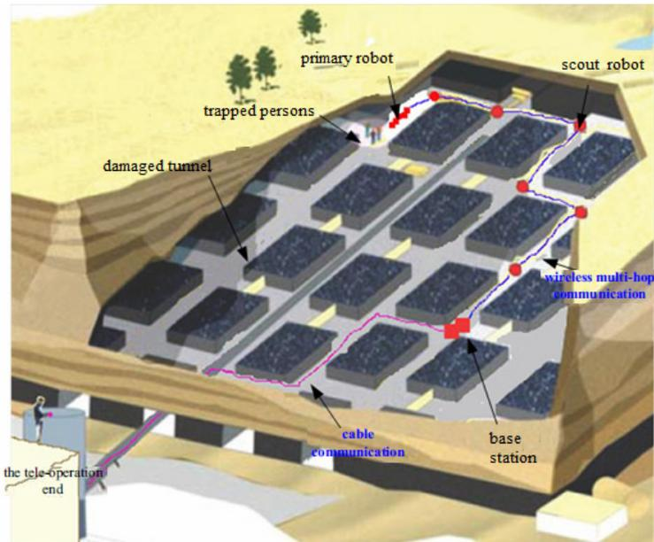
Fig. 4. The chain-topology of the multi-hop communication network
