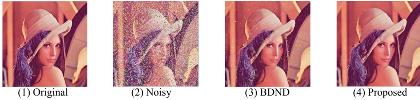
Fig. 7. Outputs for Lena (color) image for noise model 2 (40% impulse noise density {high density=30, low density=10}, m=30 )
