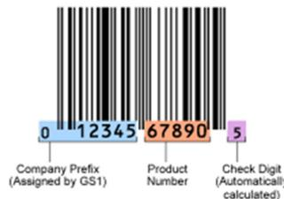
Out of the total 12 digits encoded, the company prefix can be 6 to 10 digits long
