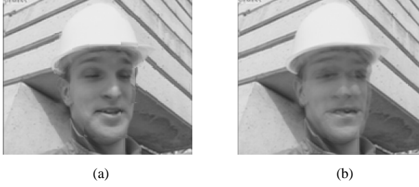
Fig. 2. The 2nd frame of Foreman sequence (30Hz, QCIF): (a) SI without SMVS (PSNR: 31.27dB). (b) SI with the SMVS method (PSNR: 31.3dB)
